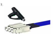
Shrink tubes - shrinking temperature 110°C.
