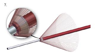
Prepare shield braid for cutting. Completely widen braid. Push outer cone (5) completely under shield braid
