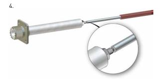
Solder contact (8) on conductor
