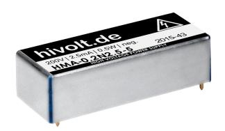
The HMA series is a line of small DC to HV converters providing 200Vpc to 1000Vpc, positive or negative, at 0.5W or 1W output power. The output voltage control is achieved by means of a programming resistor or a control voltage. An output voltage monitor and an On/Off input are provided. The units are housed in a compact PCB mountable package. The metal box and a patented resonant converter principle guarantee very low EMI. Protected against overload and short circuit. RoHS compliant.
