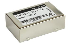
The HM36 Series is a family of ultra compact high performance - high voltage DC to DC converters with 24V supply voltage and 3W output power. Designed for PMT applications these converters are equally suitable for other applications requiring low ripple, noise and high stability. They are encapsulated in a metal package providing 6-sided shielding.
