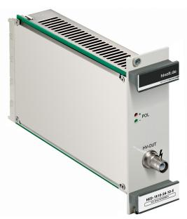
HED modules are highly precise and highly stable analog controlled high voltage power supplies with reversible output polarity. The HED series covers output voltages of up to 6 kV in a 3U/8HP cassette. A version in a compact metal box is available too (HMD series). The maximum output power is 12W
