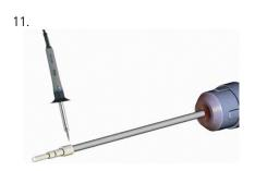
Solder contact (6) on conductor.
