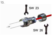
Screw cap (1) onto housing (3).
