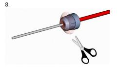
Cut shield braid to final length as defined in step 9.
