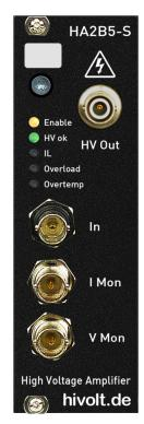
The **HA2B5-S** is a high precision high voltage amplifier 3U / 8HP / 220mm plug-in card. It provides output voltages between -2000V and +2000V at  $\pm 5$ mA. The amplifier output is available via an SHV connector located on the front panel.
