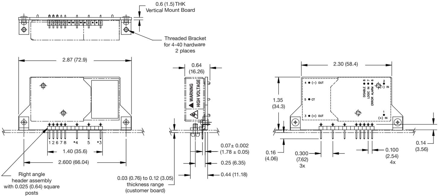
This FS-VM adaptor board provides a convenient way to mount any FS Series high voltage power supply DC to high voltage DC converter on its side, minimizing the X-Y footprint to conserve board real estate. Please note when ordering, the FS Series unit is not included and must be ordered separately.
