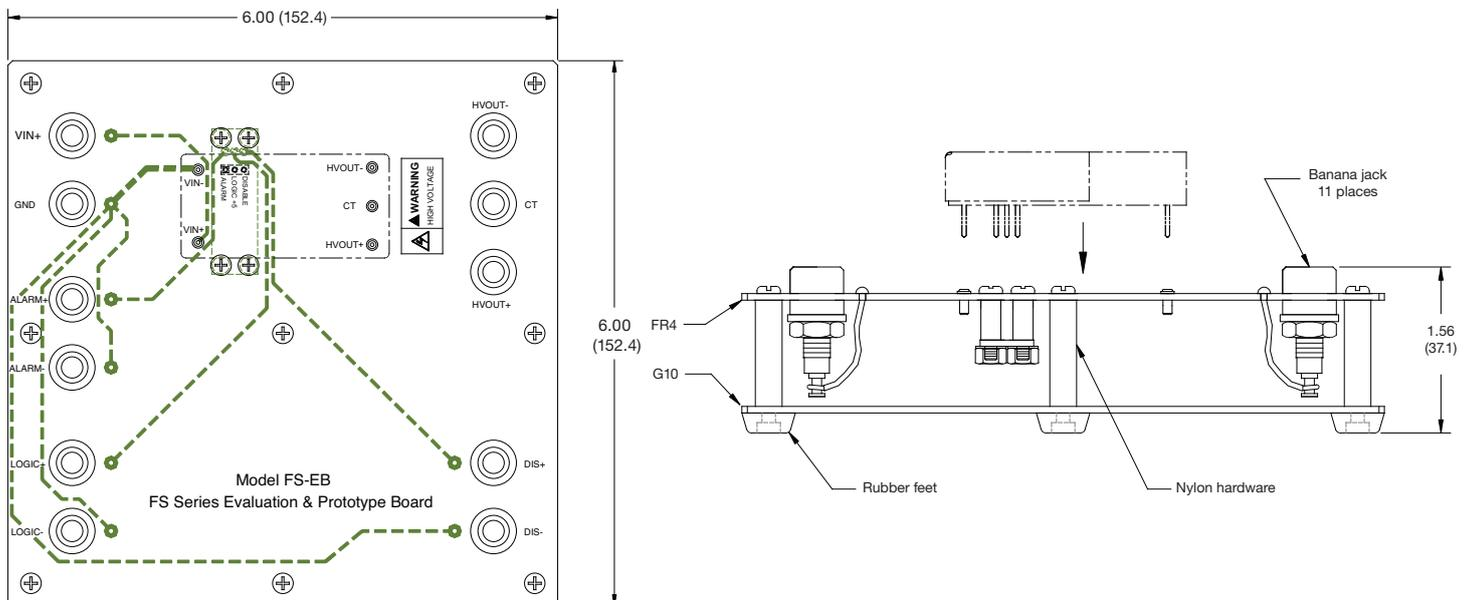
This FS-EB evaluation board provides a convenient package to use any FS Series high voltage power supply without having to fit it onto a PC board. The board provides for easy prototyping and evaluation. Please note when ordering, the FS Series unit is not included and must be ordered separately.
