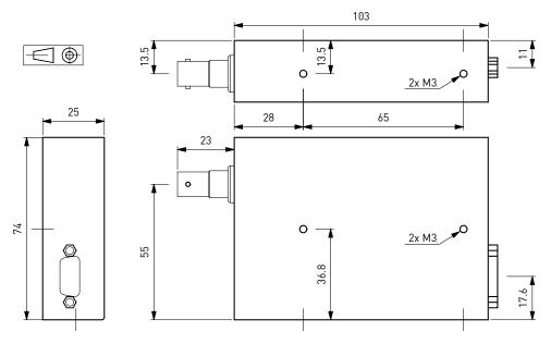
Screw-in depth of mounting screws: 5mm Dimensions in mm; drawing not to scale.
