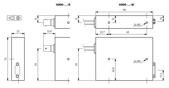
Screw-in depth of mounting screws: 5mm
