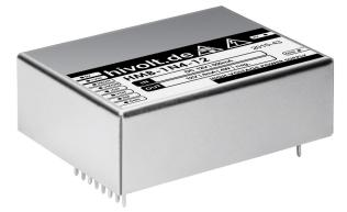
The HMB series is a line of small DC to HV converters providing 500V<sub>DC</sub> to 6000V<sub>DC</sub>, positive or negative, at 4W output power. The output voltage control is achieved by means of a potentiometer or a control voltage. The programming potentiometer can utilize the reference voltage output of the module. Output voltage and output current monitors as well as a remote ON input are provided.
