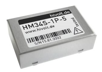
The HM34S Series is a family of high performance high voltage DC to DC converters. The converters' outputs feature protection against electric shock according to EN 61010-1:2010 / IEC 61010-1:2010-06 Edition 3.0 when connected to accessible parts. The short circuit output current is being limited to < 2mA under normal condition and < 15mA under single fault condition. The stored charge is <  $45\mu$ C.
