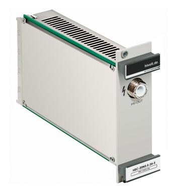
The HEC modules are highly stable, analog controlled high voltage power supplies with fixed output polarity. The HEC series covers output voltages of up to 30kV in a 3U cassette. A version in a compact metal box is available too (HMC series). The maximum output power is 12W.
